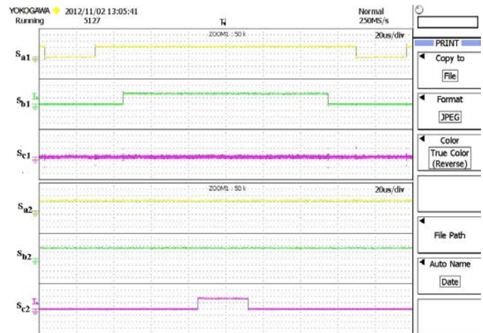
Fig. 8: Switching signals for sector-1 of phase-a, phase-b and phase-c: (a) Region-1 (b) Region-2 (c) Region-3 and (d) Region-4
